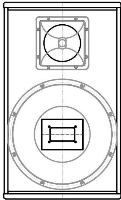
Equipped with one 15" speaker from Lavoce Italiana in a tuned enclosure. The HF section features one 2" compression driver from Celestion coupled to a diffuser, offering a dispersion of 90°x50° (H x V).
